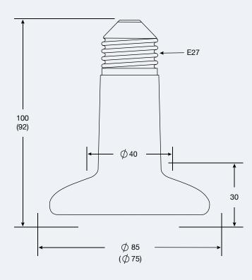
Figure 2: Mounting dimensions and radiator dimensions () in mm
